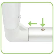
2. Push snap buttons and slide into hole to secure.
