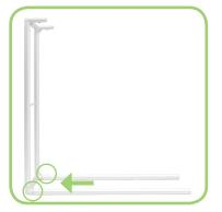
**1.** Slide the bottom horizontal tubes onto the side of frame.
