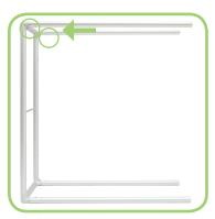
**3.** Slide the top horizontal tubes onto the side of frame.
